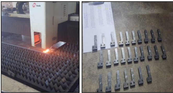
Fig -4: Manufacturing of Jobs on Laser Cutting Machine
