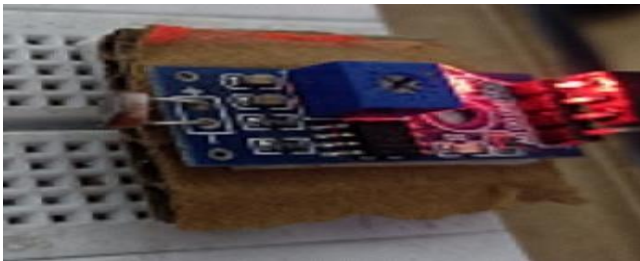
Fig. 3.1. The LDR module used in the project.
