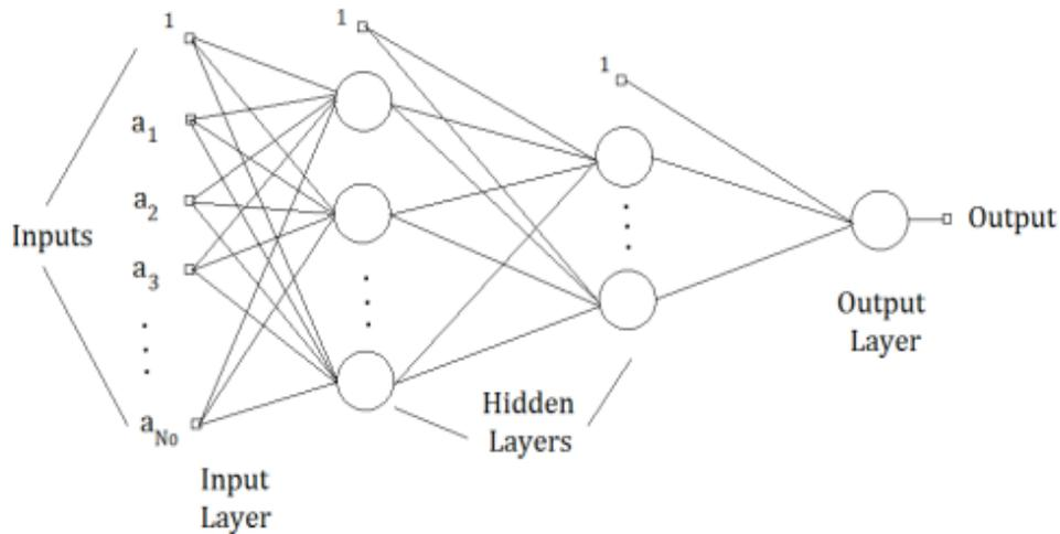
Figure 1: A basic three-layer architecture of a feed forward ANN.
