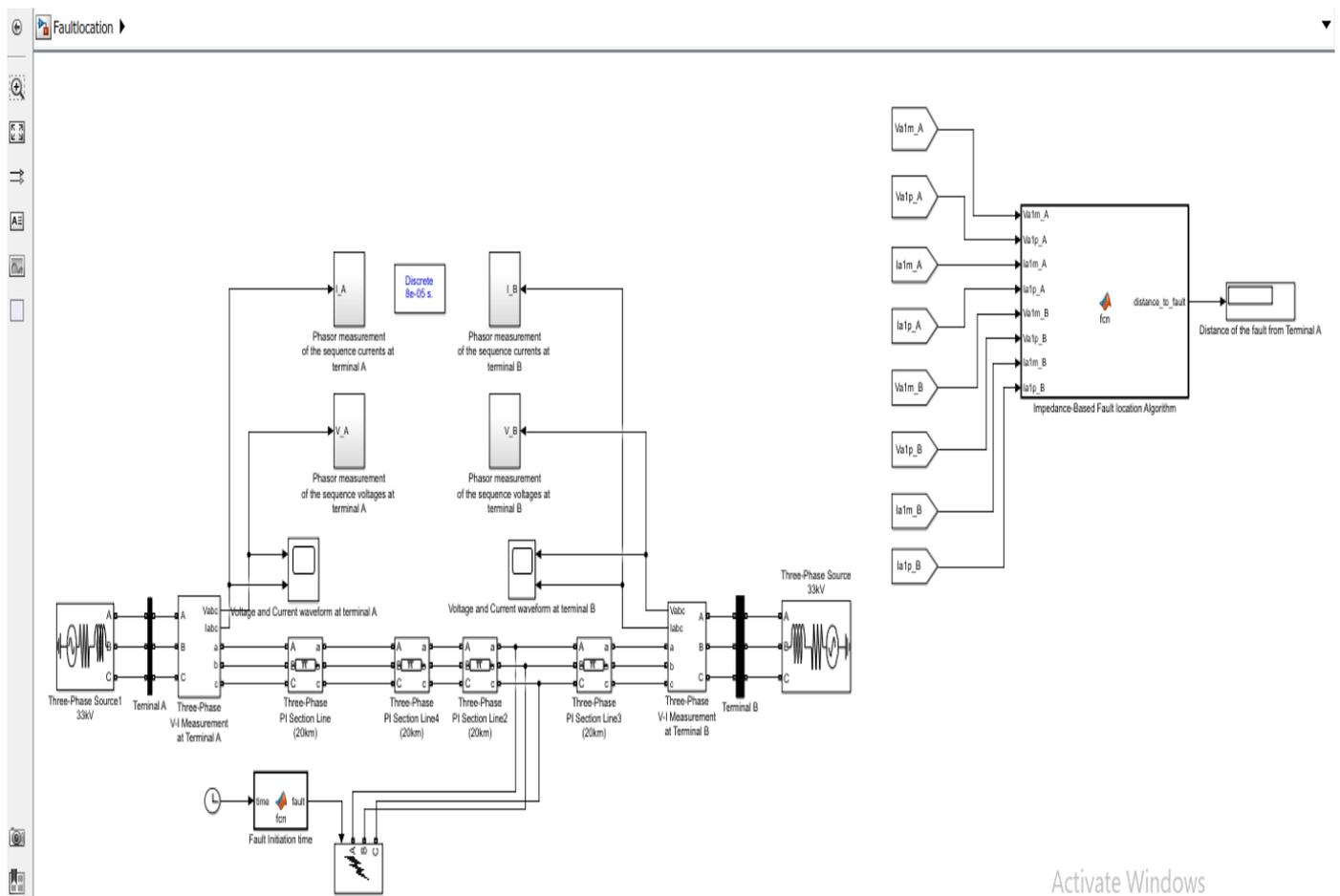
Based on the above simulink diagram the fault location is calculated by placed the fault between the phase A and B , By changing the line length of the transmission line the fault location will change accordingly with reference to A. The fault location time is set at 0.2 sec, so in the current and voltage graph , it shows changes from time 0.2 seconds.
