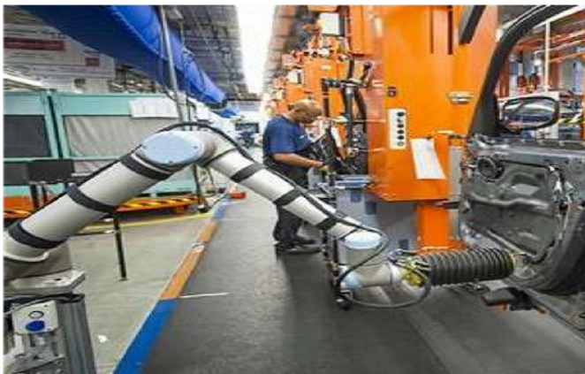
Fig 4. Cobot helping in the door assembly operation in BMW plant of South Carolina. [10]
