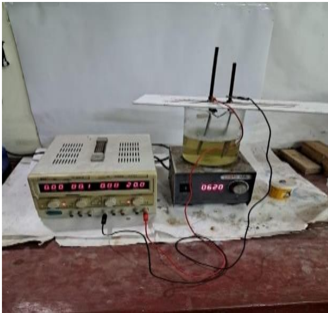
Fig 2: Experimental set up by Electro Electrocoagulation
