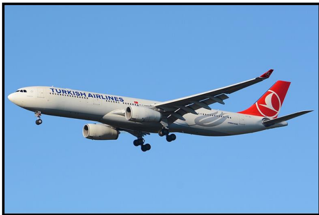
Fig 22 : Airbus A330, one of the most used Commercial Aircraft which uses Supercritical Airfoil
