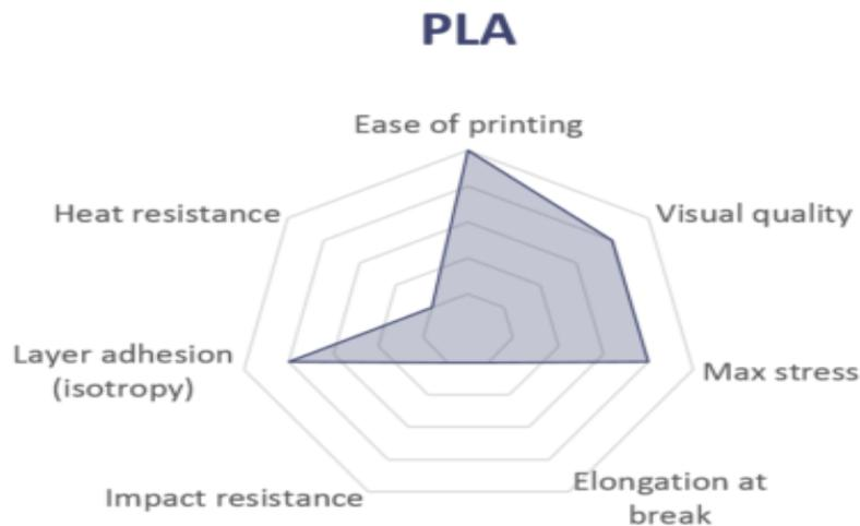
**Figure 3** The material profile of PLA
