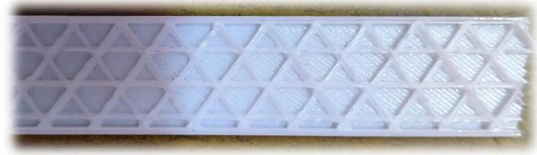
Figure 9 shows the Cubic-Subdivision Infill Pattern
