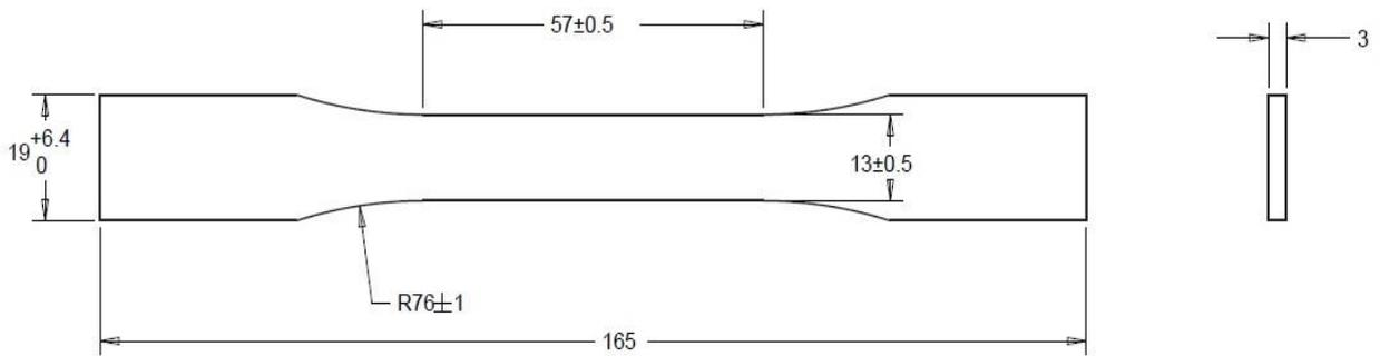
Figure 10 Specification of the specimen
