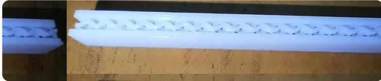
Figure 8 shows Gyroid Infill Pattern
