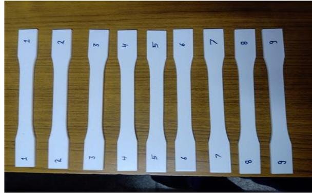
Figure 11 FDM fabricated specimens
