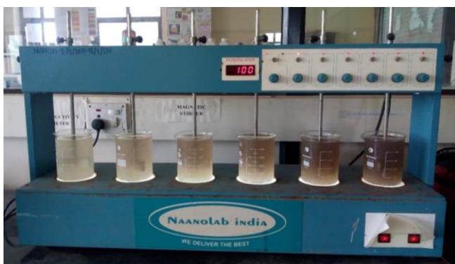
Fig - 7 Jar Test Using Natural Coagulant CARICA PAPAYA L (Papaya Seeds)
