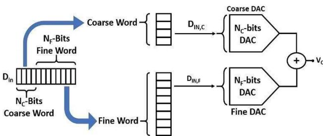
Figure 4 - Segmented DAC Architecture:
