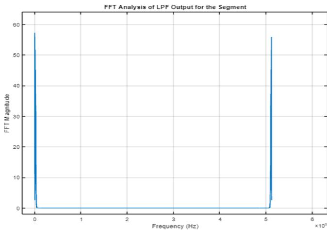
Figure 8 - FFT Analysis of Segmented 16-bit DAC Output
