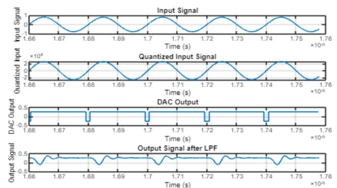
Figure 5 - 16-bit Sigma Delta DAC Output
