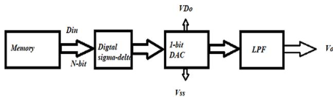
Figure 3 - Sigma-Delta DAC Architecture
