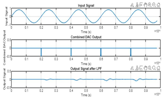
Figure 7 - Segmented 16-Bit Sigma Delta DAC Output
