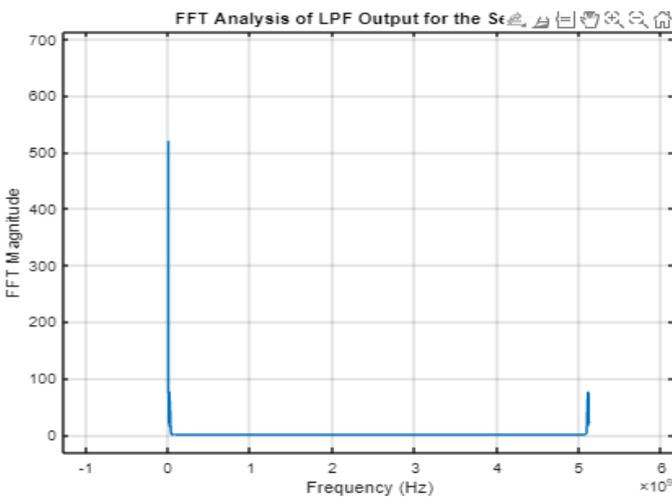
Figure 6 - FFT Analysis of 16-bit DAC Output
