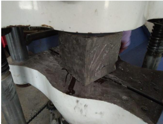
Compressive strength test
