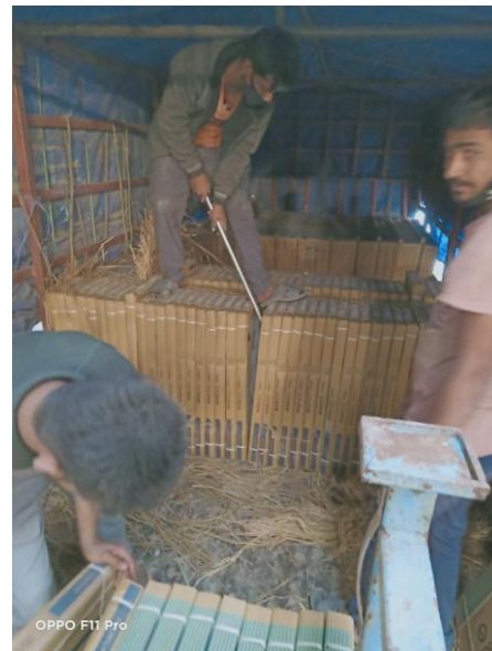
Fig – 5 - Tighten the rows to avoid Breakage
