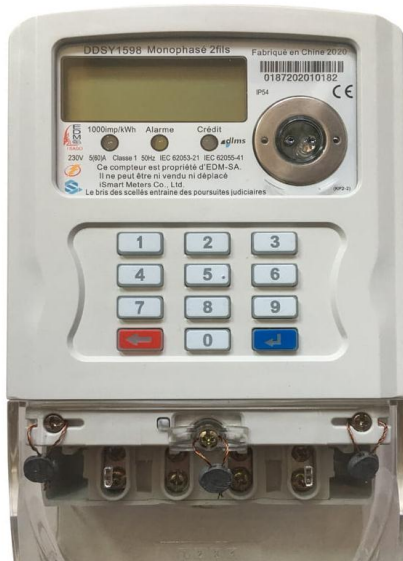
Figure 1.1 Prepaid energy meter
