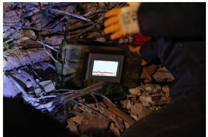
Figure 9 : The Through The Wall Radar (DAR) produced by STM[18]
