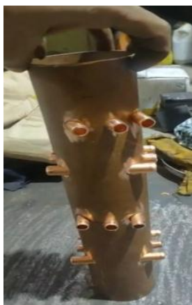
Fig -2: Modified core section of vessel
