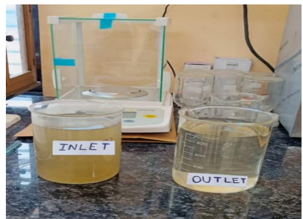
Fig - 7: Sewage Treatment Plant Inlet and outlet Water Sample
