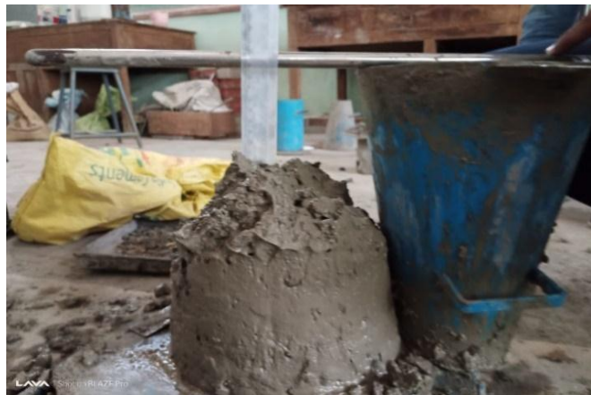
Fig- 6: Slump cone test
