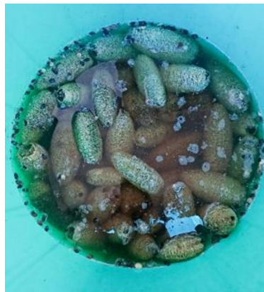
Fig-3: Loofah Fiber Soaked in the Solution
