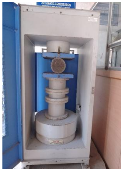
Fig.-4: Testing of Specimen for Split Tensile Strength
