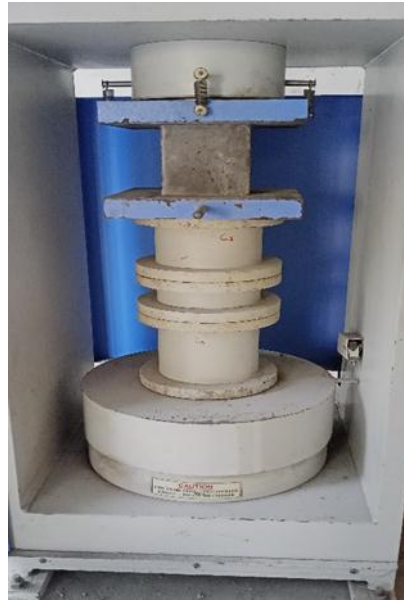
Fig.-4: Testing of Specimen in Compression Testing Machine
