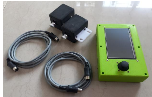
Fig -2: Auto-Stellar Motor Drive & Controller Setup with Motor Cords
