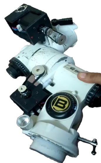
Fig -3: Equatorial Mount with Motors.
