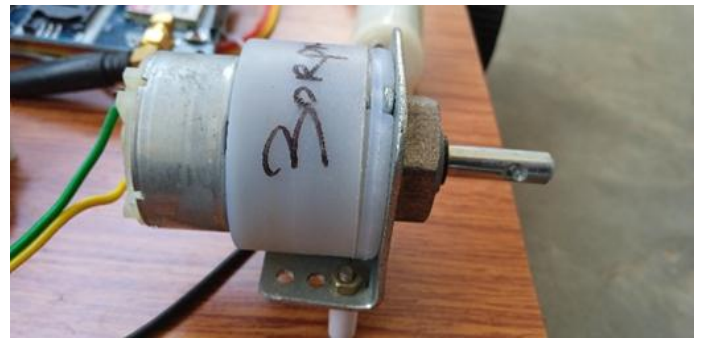
FIG-6: DC Motor ( Fire Extinguisher Ball )
