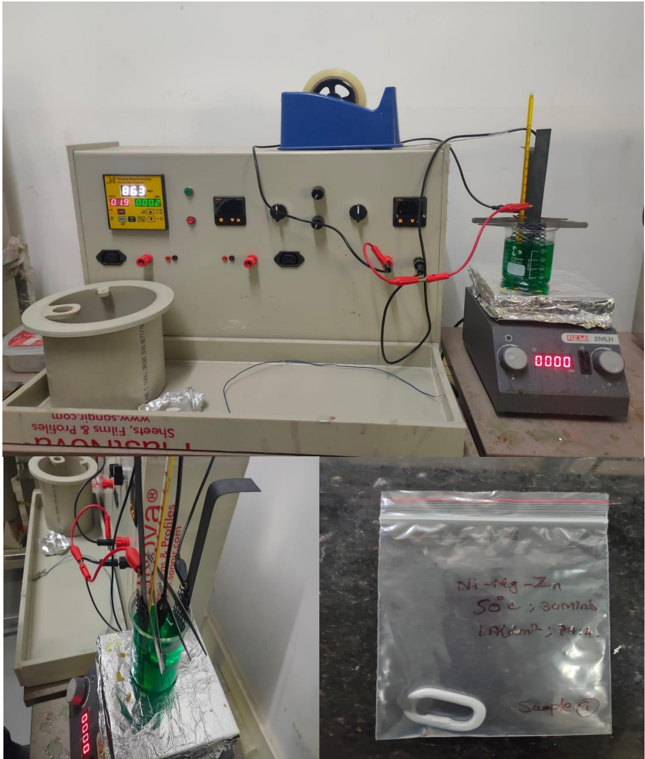
Fig-1 : Electrolytic Bath Composition of Ni-Mg-Zn
