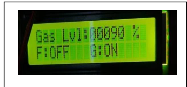
Fig-15: Shows the reaction on detection of Gas leakage.
