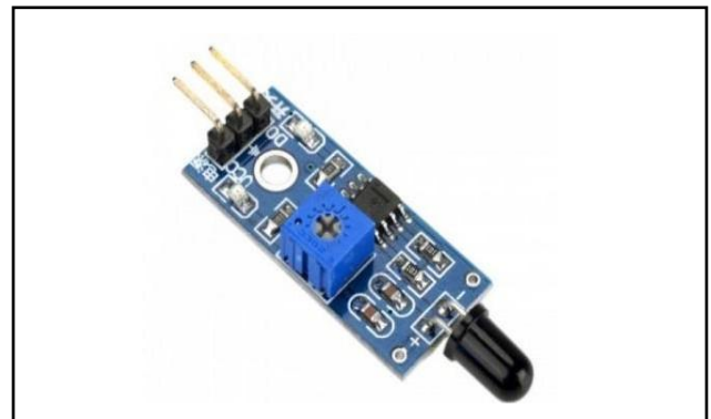
Fig-7: Flame sensor for Fire detection
