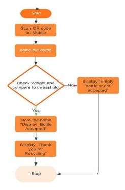
The bottle may be put into the chamber once the user scans the displayed QR code. If the bottle weighs less than the predetermined amount, it is taken inside the chamber and the message "BOTTLE ACCEPTED" is shown. The word "THANK YOU" is displayed to show how much are appreciated for their contribution to the recycling process. The bottles are rejected and labelled "EMPTY BOTTLE" if the weight of the bottle measured is more than the pre-set value.
