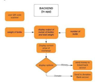
When the user scans the QR code once it has been presented, the machine dispenses the bottle and measures its weight and sends rewards accordingly to the mobile application which can further be redeemed for physical money.
