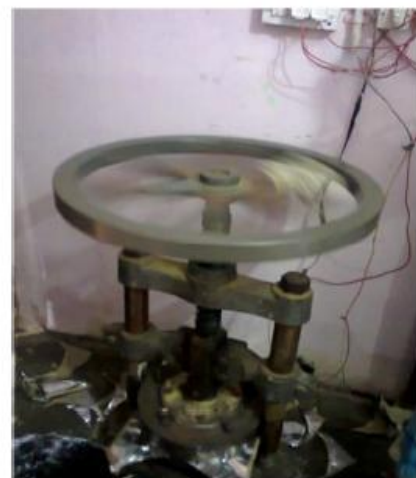
Fig.5.1.2 Image of manually operated press machine.
