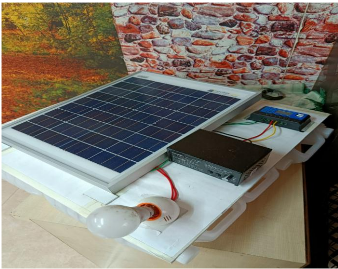
Figure 5 a prototype of floating solar plant of 20 w capacity with recycled plastic cans
