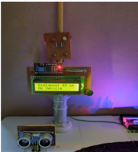
Fig -14: LCD display working
