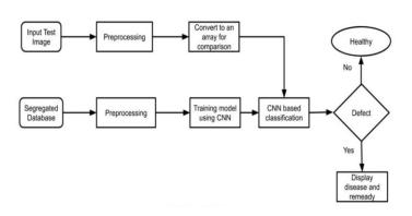
The proposed system of automatic and reliable pomegranate leaf disease detection using AlexNet is a deep learning-based approach that can accurately detect and identify the type of disease affecting the leaf. The system consists of three main steps:
