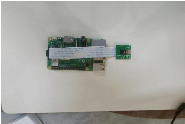
Fig-2: Camera Sensor connected with Raspberry Pi
