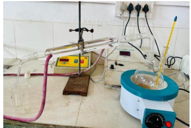
Fig. Experimental setup for simple distillation (Purify oil)
