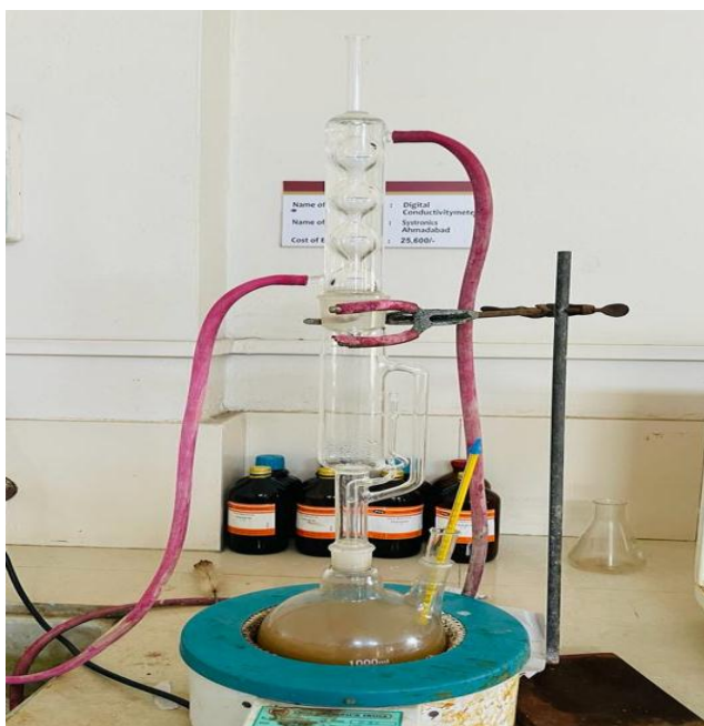
Fig. Experimental setup for extraction of oil
