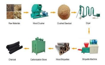
**Preparation of raw materials :** The first step is to collect the raw material, which can be agricultural waste, sawdust, wood chips, or charcoal dust. The raw materials is then dried to reduce its moisture content, which is important for achieving high quality briquettes.
