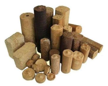
Raw material selection: Choosing the right raw material is crucial for producing high quality biomass briquettes. It's important to select materials that have consistent size, low moisture content, and high calorific value to ensure optimal combustion efficiency and reduce waste.
