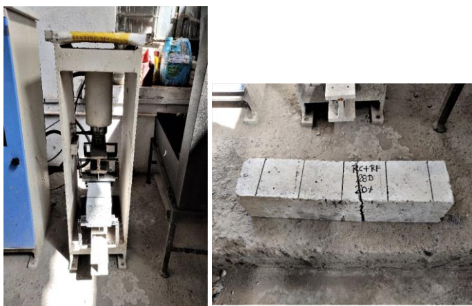
Fig. 3. Testing of flexural strength sample using flexural strength setup on compressive strength testing machine
