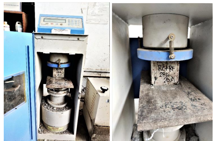
Fig.1. Compressive Strength Test of Cube
