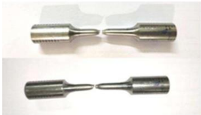
Fig -3.2: Failure Specimen
