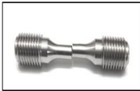
Fig -4.2: UNS S31803 un-notched specimen after failure
