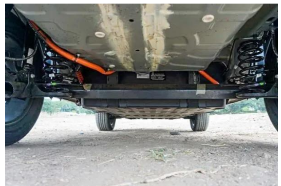
Figure 11 Tata Nexon EV max undertray
