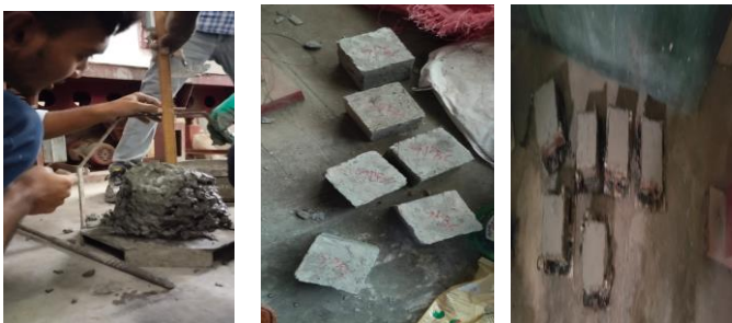
Fig 2. Prepared Specimens - Marking of Specimen ID and GPC Specimens under ambient curing
