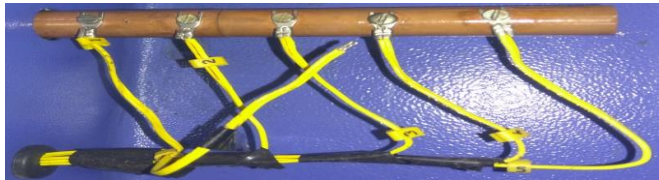
Fig 2.6 (d): Copper coated over Aluminium Pin Fin Table-2: Experiment Readings under Natural Convection
