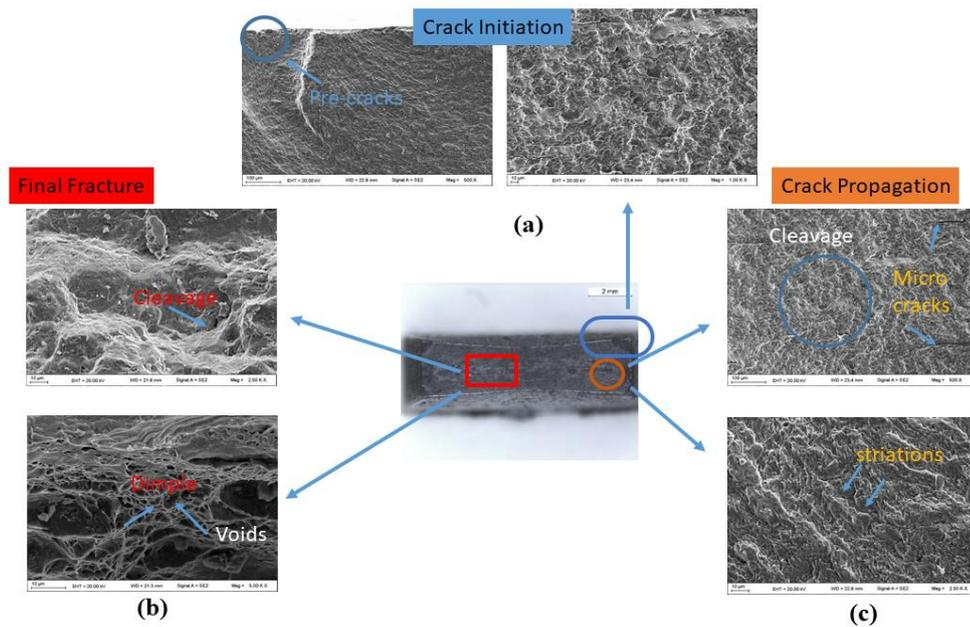
Fig.6 SEM micrographs, fracture surface after HCF testing at 50% load
