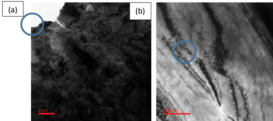
Fig.8 TEM micrographs, fracture surface after HCF testing (a) fracture zone at high stress amplitude (b) pearlite phase presence; dark field image (in a circle)
