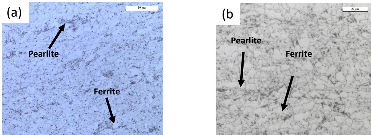
Fig.2 Optical micrographs of as received sample at different magnification
