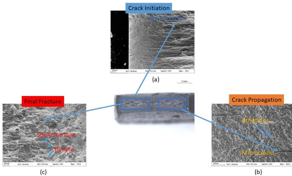
Fig.7 SEM micrographs, fracture surface after HCF testing at 90 % load
