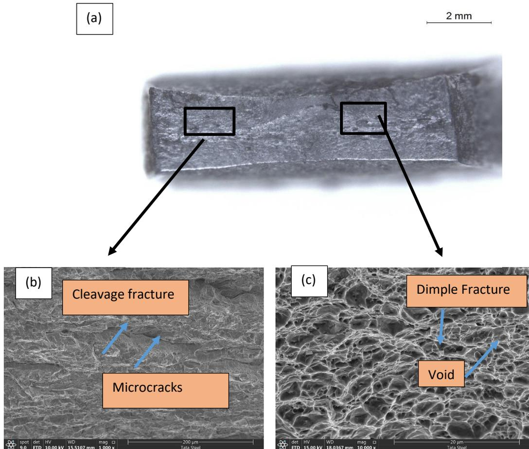
Fig 4. SEM Image tensile tested specimens at different magnifications
