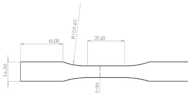
Fig.1 Schematic diagram of High cycle fatigue specimen
