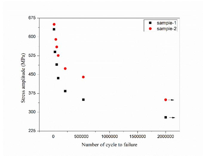
Fig.5 Stress life curve. Data point with arrow indicate no failure
