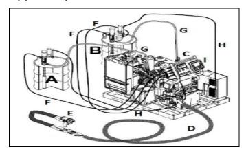
The diagram depicts a set of machines for spraying polyurea coating or foams, including a combustion engine, electricity generator, and air compressor, enabling real-time control of mixture parameters.
