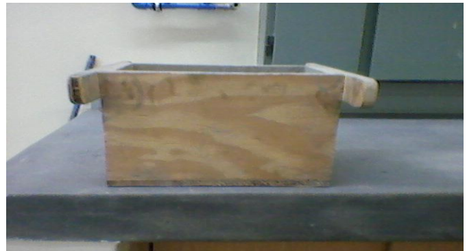
Fig. 3: Constructed gauge box for volume batching
