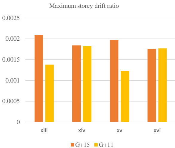
Chart-9: Variation of Maximum Storey Drift Ratio for cases xiii to xvi
