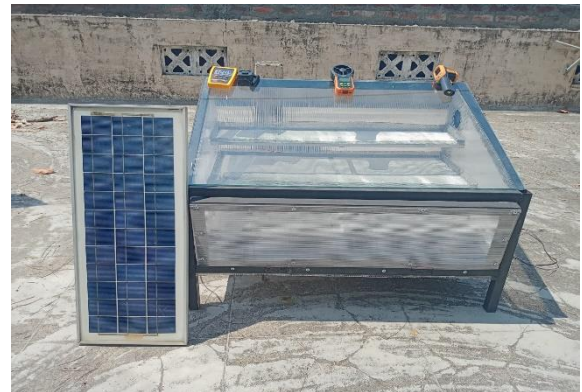
Figure 1. Computerized representation and photographic view of the direct solar dryer.
