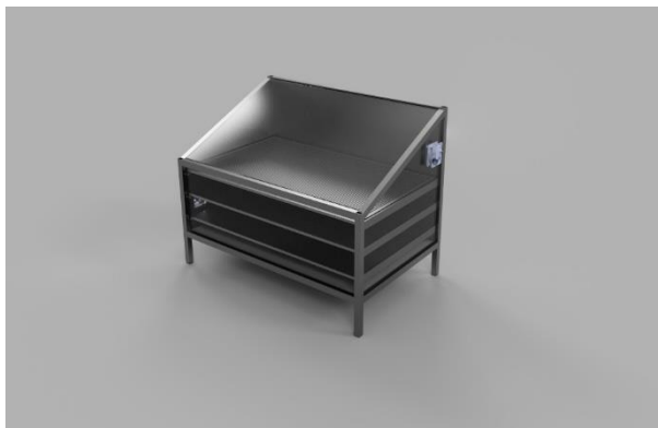
Figure 1. Computerized representation and photographic view of the direct solar dryer.
