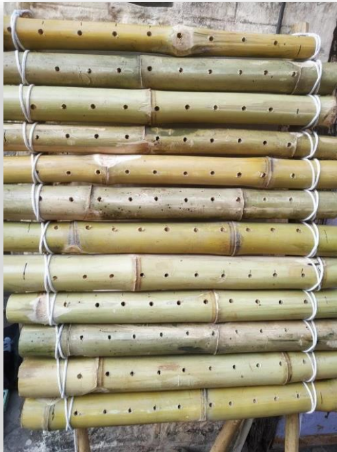
Fig -2: Bamboo Panel with full bamboo poles
