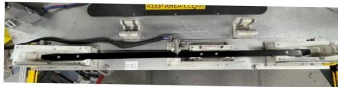
Fig -2: Roof rail on jig fixture without stanchions
