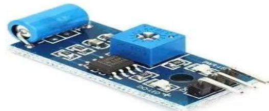
Figure-5: Vibration sensor
