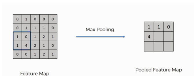
Fig- 6: Example of max pooling
