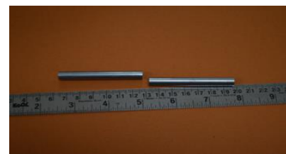
Fig 3. SS321 Pipes ready for welding process
