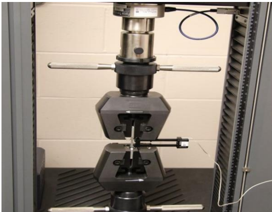
Fig 11. Universal Testing Machine pipes gripped in chucks
