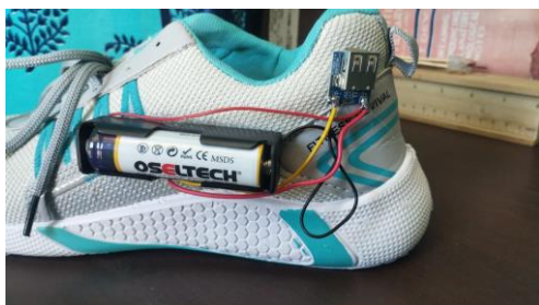
Fig 5 : Side View of shoe (PCB attached to charge USB devices)
