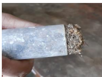
Fig-8: Removing the stabilized sand samples from the mold pipes
