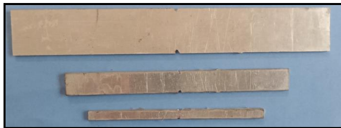
Fig -2: specimen with center double-edge notch
