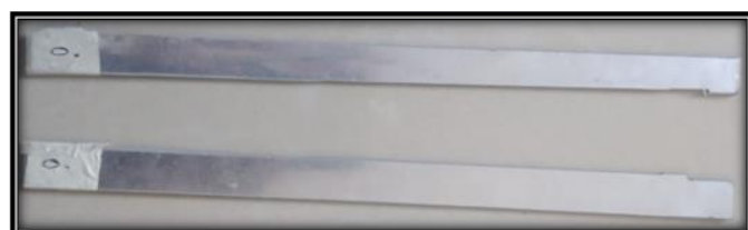
Fig -1: Specimen (0°fiber direction)
