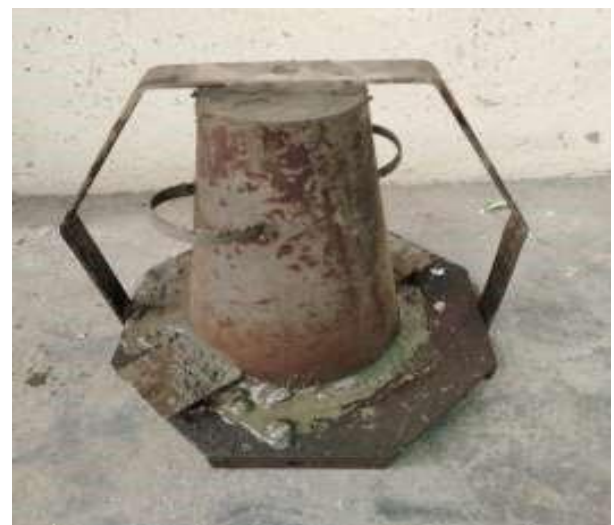
Fig-9: Slump test
