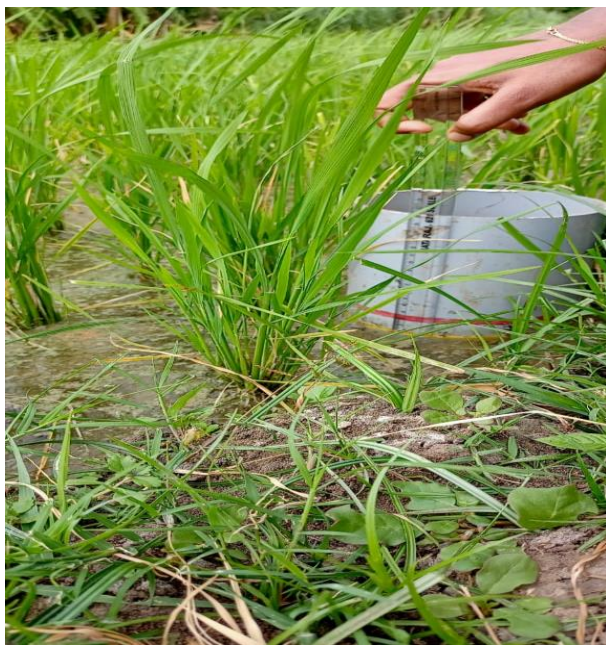
Fig 2.2 Measuring water Level inside Pani pipe
