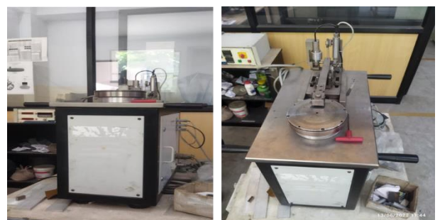
Fig 5.6 Pin on disc testing apparatus
