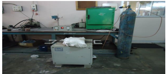
Fig 5.3 Experimental Setup for stir casting furnace
